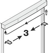
**4.** Transfer lower hinge bracket and cover plate to the opposite side.
