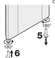
**5.** Turn lower hinge pin through 180° and remove.
